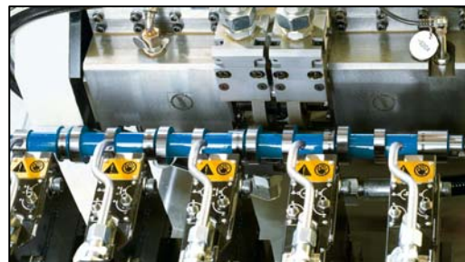
Grinding station 2: Pair-wise grinding of cam pairs
