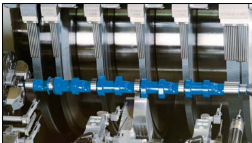
Grinding station 1: Grinding of bearing and pivot diameters
