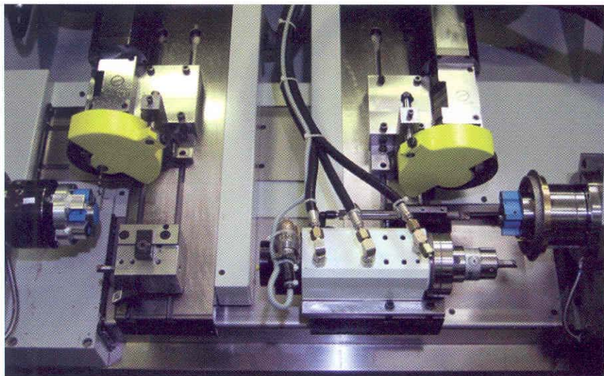
Junker's slant bed design uses a flexible gang tool carrier to bring turning, milling and grinding tools into the cutting zone. The grinding modules (seen with yellow wheel guards) can be fitted with drills for hard drilling operations.
